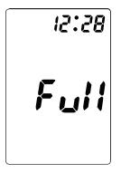
When the memory is full the LCD screen of the device displays 'Full' and no further measurements or medication records can be performed. Upload the measurement data and clear the memory to reset the device.
