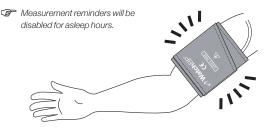
Five seconds before the next scheduled measurement, the device can emit a short series of beeps to notify the patient of the coming measurement (optionally). The beep is switched off by default and can be enabled via software setting. (See instruction manual of the WatchBP Analyzer)
